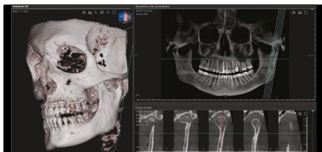
SUPERIOR CONFIGURATION Together with the Essential configuration, the Superior FOV range extends the scope for treatment to the gnathology, otolaryngology and the maxillofacial field, including scans of both adult temporomandibular joints. • FOV: 13x16; 15x6; 15x10; 15x16
