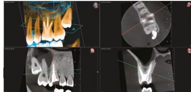
ENDO PACK For endodontic and implantology analysis at maximum resolution, reaching 50 µm (Voxel). Limits the area exposed to X-rays and so minimises the emitted dose, most importantly with paediatric patients. Optional pack that can be paired with the Essential and Superior configurations.
